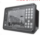
The Stratomaster is a comprehensive flight, engine and navigation instrument designed for Experimental and Light Sport aircraft. The large amount of flexibility built into the base system allows the adaptation of the Stratomaster to almost any mission and aircraft. Due to low system cost, Stratomaster is equally suited to very light aircraft, gliders and rotorcraft, while providing enough flexibility to be utilized by even twin-engine aircraft with
