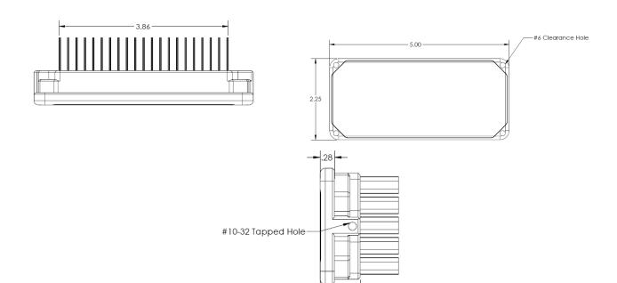
Voltage Range: 9-36VDC Height: 2.25" Current Draw at 14VDC: 2.6 Amps Max Width: 5" Power Consumption: 36 Watts Max Depth: 1.5" Weight: 8 Oz Pulse Light Feature: Built In
